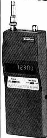
IM-2400 Hand-held Frequency Counter. Measures 50Hz to 512MHz in two ranges. 7 digit LED Display. Crystal-controlled 10MHz time base. Operates on nickel-cadmium batteries or line current with optional eliminator charger. Swivelling Telescopic Antenna optional.
