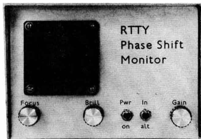
Front view. Actual size 3.5 by 5in with 2in crt. The switch marked "in-alt" allows for switching an "alternative" input from a second receiver. This is not shown on the circuit diagram, and may be omitted
